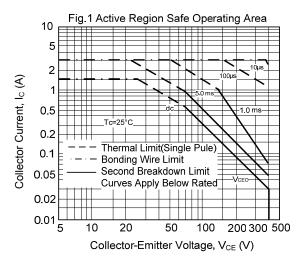
The Safe Operating Area of Fig.1 are specified ratings (for these devices under the test conditions shown.)
