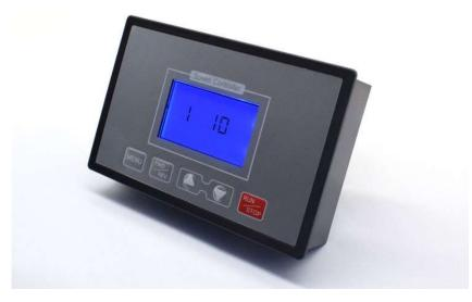
Slow stop time setting Press the MENU button 3 times to enter the function 2 setting key surface Press the plus and minus keys to set the time Press RUN/STOP to save and exit (10 is 1 second, 100 is 10 seconds)
