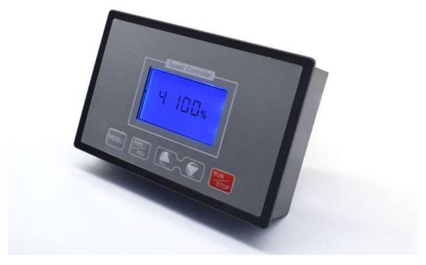
Set acceleration and deceleration value Press the MENU key 6 times to enter the function 5 key surface Press the plus and minus keys to switch Press RUN/STOP to save and exit
