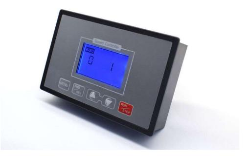
Slow start time setting Press the MENU button 2 times to enter the function 1 setting key surface Press the plus and minus buttons to set the time Press RUN/STOP to save and exit (10 is 1 second, 100 is 10 seconds)
