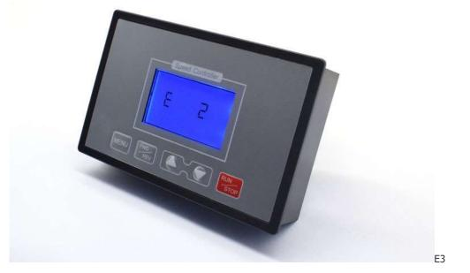
function: according to the starting motor forward rotation, forward rotation to positive limit motor reverse rotation, reverse rotation to reverse limit motor stop
