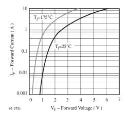
Figure 4. Max. Forward Current vs. Forward Voltage
