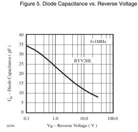
Figure 6. Diode Capacitance vs. Reverse Voltage
