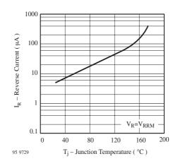
Figure 2. Max. Reverse Current vs. Junction Temperature
