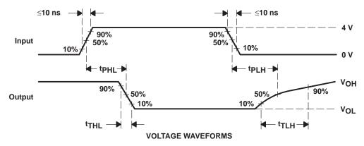
NOTES: A. The pulse generator has the following characteristics:  $Z_0 = 50 \Omega$ ,  $t_W = 500 \text{ ns}$ .
