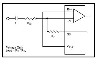
Figure 6 - Single-Ended Input Configuration
