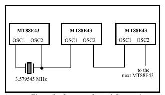
Figure 8 - Common Crystal Connection
