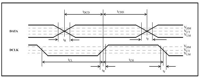
Figure 12 - DATA and DCLK Mode 0 Output Timing
