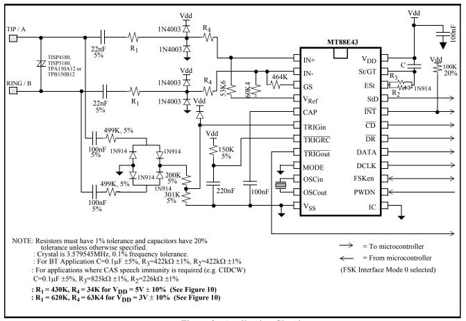
Figure 9 - Application Circuit
