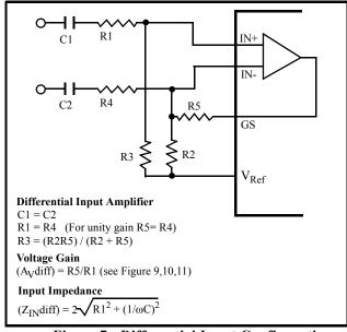
Figure 7 - Differential Input Configuration
