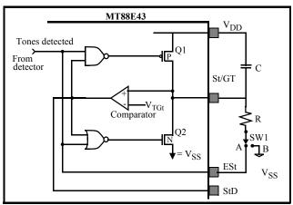
Figure 4 - Guard Time Circuit Operation
