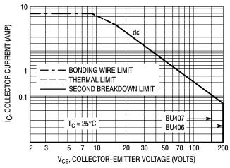
Figure 2. Maximum Rated Forward Bias Safe Operating Area
