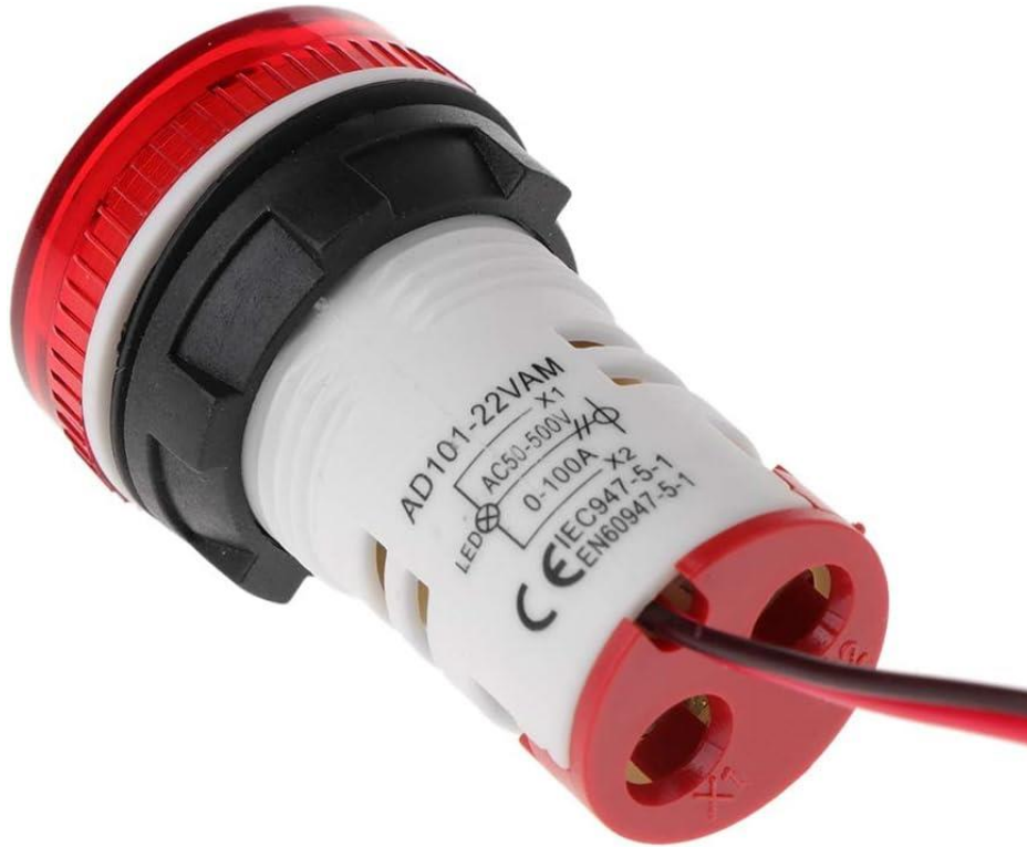
Figure 2: Rear view of the voltmeter ammeter, illustrating the wiring terminals for power input and current transformer connection. Note the AD101-22VAM model designation and AC50-500V, 0-100A ratings.
