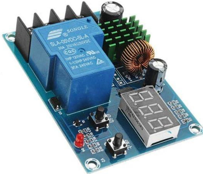
Figure 1: XH-M604 Module with labeled components. Key components include the voltage display digital tube, starting voltage setting button, stop voltage setting button, and output indicator lamp.
