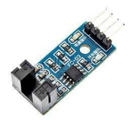
Widely used in motor speed detection, pulse count, the position limit, etc. The DO output interface can be directly connected to a micro-controller IO port, if there is a block detection sensor, such as the speed of the motor encoder can detect.
