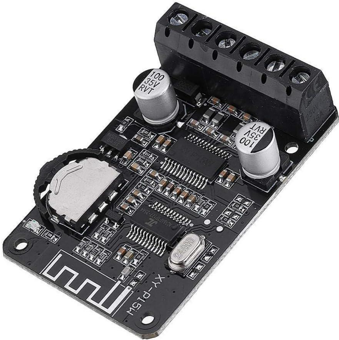
Image 1.1: Top view of the DollaTek XY-P15W Bluetooth Amplifier Module, showing the main components and terminal blocks.
