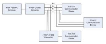
(2) When the HXSP-2108B connects as RS-232/RS-4485, the device connects as RS-485 connection method.
